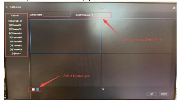
3. The same channel number cannot appear in the same layout box, but multiple channel numbers can appear in the one layout box.
